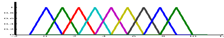
Fig (ii), First degree B-spline basis function with uniform Knot vector X = \{-1, 0, 1, 2, 3, 4, 5, 6, 7, 8, 9, 10, 11, 12\}
