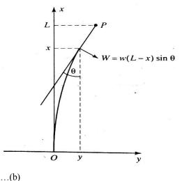
Now make the approximation that the deflection at point x on the rod is small, so  $\sin\theta = \tan\theta = \frac{dy}{dx}$ From (a),(b),(c) we arrive at third order differential equation
