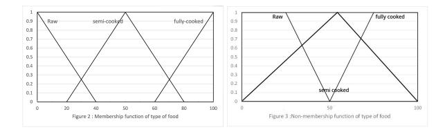
We will explain the working of the controller with an example. Let the input for the type of food and quantity of food be 65 and 75 respectively. Lets fuzzify these values using membership and non membership functions of both inputs.
