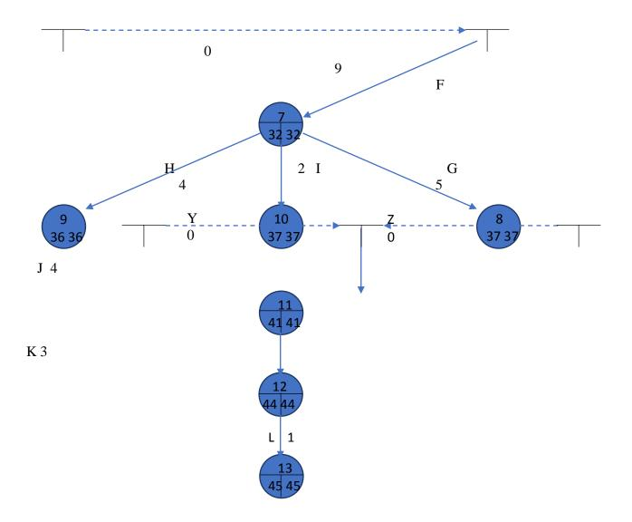
The network analysis shows the different paths available to the company to go from event 1 i.e. the start of the project to event 13 i.e. the end of the project. X, Y & Z are the dummy paths formed to meet the requirements of predecessor activities. The duration for each activity is shown besides the activity code. The tail circle for each activity shows the early start and the late start for the activity on the bottom-left and the bottom-right respectively.
