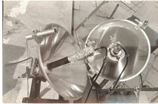
Fig. 1 Truncated cone mirror with a tubular reactor on its axis, receiving sunlight reflected by a flat plane mirror.
