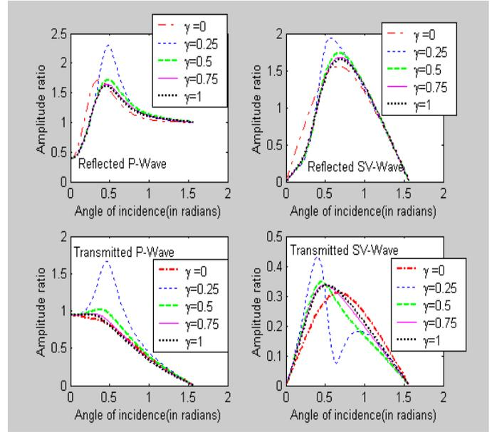
Figs. 2-5. Variation of the amplitude ratios of reflected P-wave, reflected SV-wave, transmitted P-wave and transmitted SV-wave with angle of incidence of P-wave.
