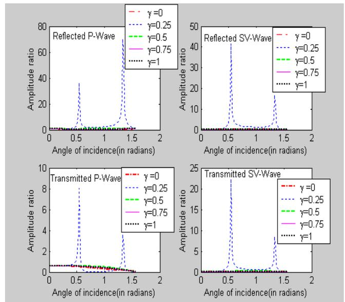
Figs. 6-9. Variation of the amplitude ratios of reflected P-wave, reflected SV-wave, transmitted P-wave and transmitted SV-wave with angle of incidence of P-wave in case of empty porous solids.
