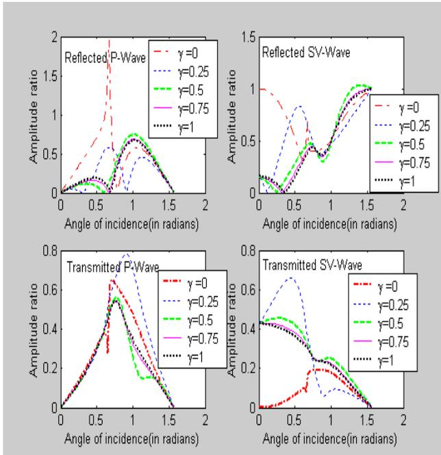
Figs. 14-17. Variation of the amplitude ratios of reflected P-wave, reflected SV-wave, transmitted P-wave and transmitted SV-wave with angle of incidence of P-wave in case of empty porous solids.
