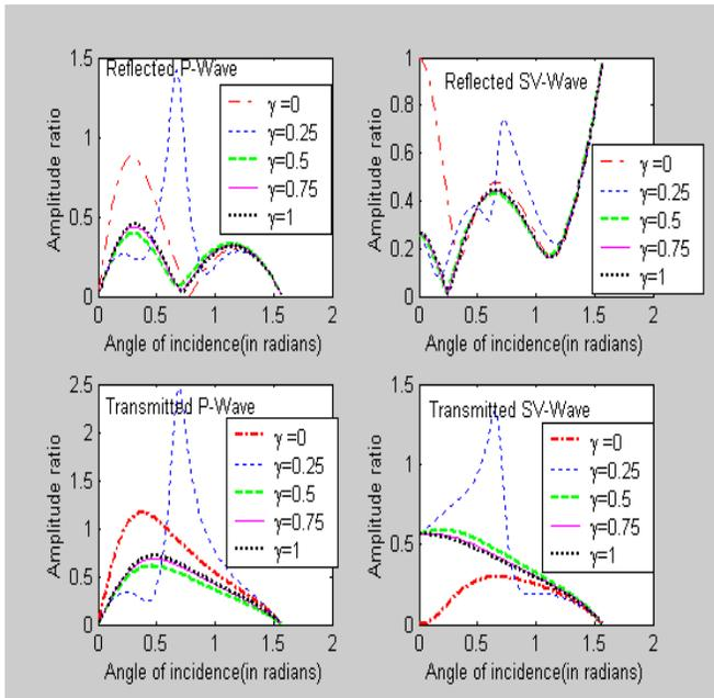
Figs. 10-13. Variation of the amplitude ratios of reflected P-wave, reflected SV-wave, transmitted P-wave and transmitted SV-wave with angle of incidence of SV-wave.
